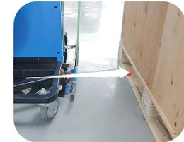
**Note :Make sure the drawing head is towards the middle of the pallet hole**
